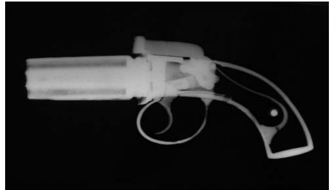
Fig. 4: Radiograph of pistol showing internal components.
