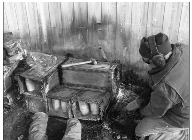
Fig. 7: Using Dynadrill to free frozen provision cases.
